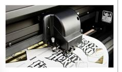
**OPOS-X** contour cutting alignment enables you to die-cut valuable printed vinyl graphics with complete confidence and reliability.
